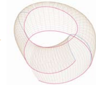
Surface Generation=Section Profiles + Plan Profiles
